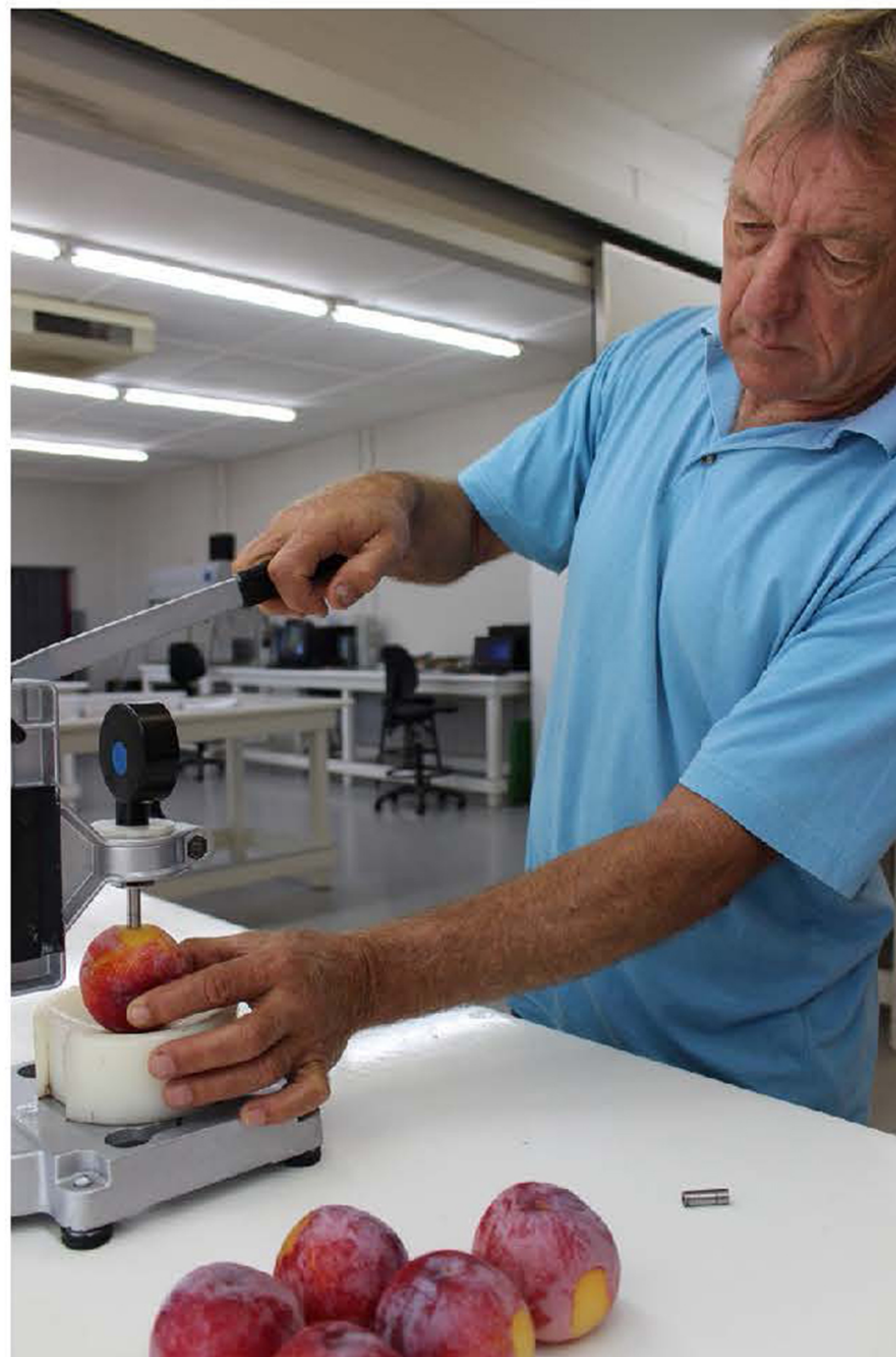
Above: Arrie de Kock demonstrates the correct use of the penetrometer during a new trial on plums.
